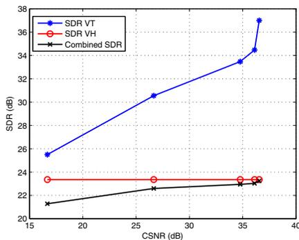
Fig. 6. SDR-vs-CSNR performance when three analog sensors (Tx) communicate simultaneously using AJSCC to a digital Cluster Head (CH), the receiver (Rx).
