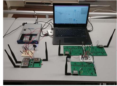
Fig. 4. **System prototype.** Three analog sensing boards (right bottom) communicating to an analog receiver (left bottom). The baseband signals of all three channels are captured using NI Digital Acquisition System (DAQ) (left top) and processed/decoded on a host laptop using LabView/MATLAB.
