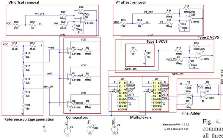
Fig. 3. **LTSpice schematic** of analog components of the second stage of the AJSCC-mapping analog circuit, where functional blocks are logically “boxed.”
