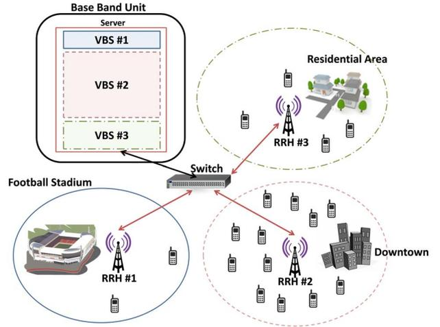
Fig. 1. Cloud Radio Access Network (C-RAN) architecture, where the Base Stations (BSs) are physically unbundled into Virtual Base Stations (VBSs) and Remote Radio Heads (RRHs). The use of virtualization in C-RAN allows for dynamic re-provisioning of spectral and computing resources based on traffic demand fluctuation.
