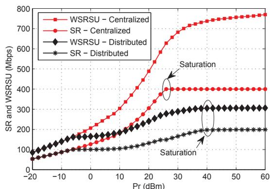
Fig. 5. Downlink WRSRU of a C-RAN system with centralized computing resource (*Centralized*) versus that of a traditional system with distributed computing resources (*Distributed*).
