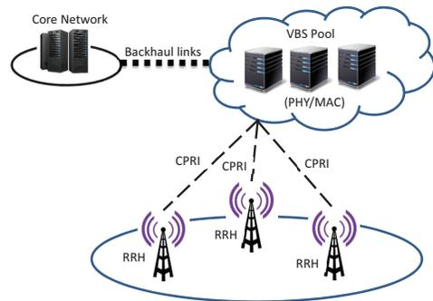
Fig. 1. Cloud Radio Access Network (C-RAN) Architecture.
