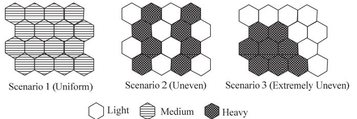
Fig. 3. Different user distribution scenarios: Scenario 1 (uniform) with all *medium* (loaded) cells; Scenario 2 (uneven), *light* and *heavy* (loaded) cells are intermixed together; Scenario 3 (extremely uneven), *heavy* cells are grouped together, and the heavy cell group is surrounded by *light* cells.
