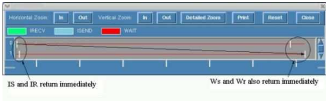
Figure 3.2: Profile of the test on MPICH where process 0 (top) sends a 1 KB message to process 1 (bottom).
