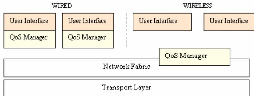
**Figure 3.3 QoS Manager in Heterogeneous Collaboration Framework**
