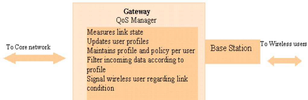
**Figure 3.4 Wireless gateway QoS Manager Functions**
