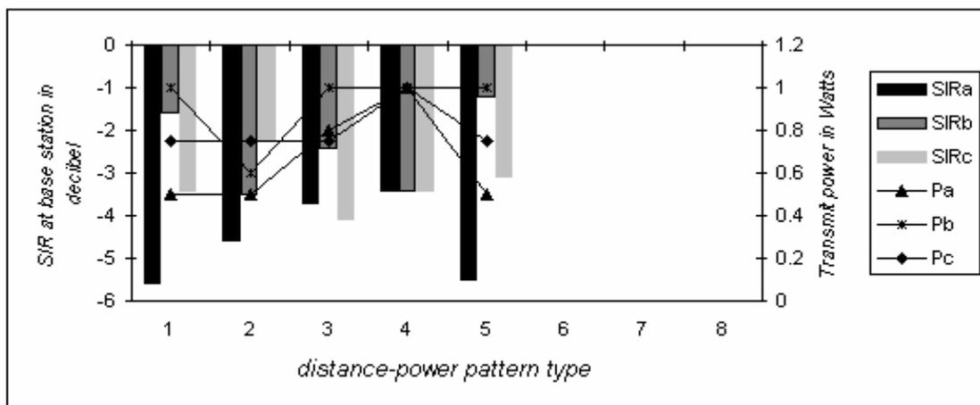
Figure 5.6 Performance of 3 wireless clients with varying distance and power
