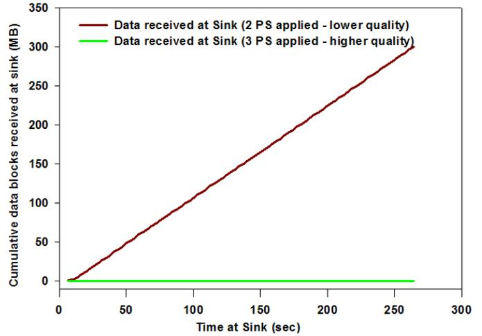
Fig. 16. Quality of data received at sink during congestion without adaptation at in-transit nodes.
