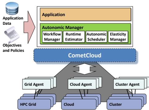
Figure 1: Architectural overview of the autonomic application management framework.
