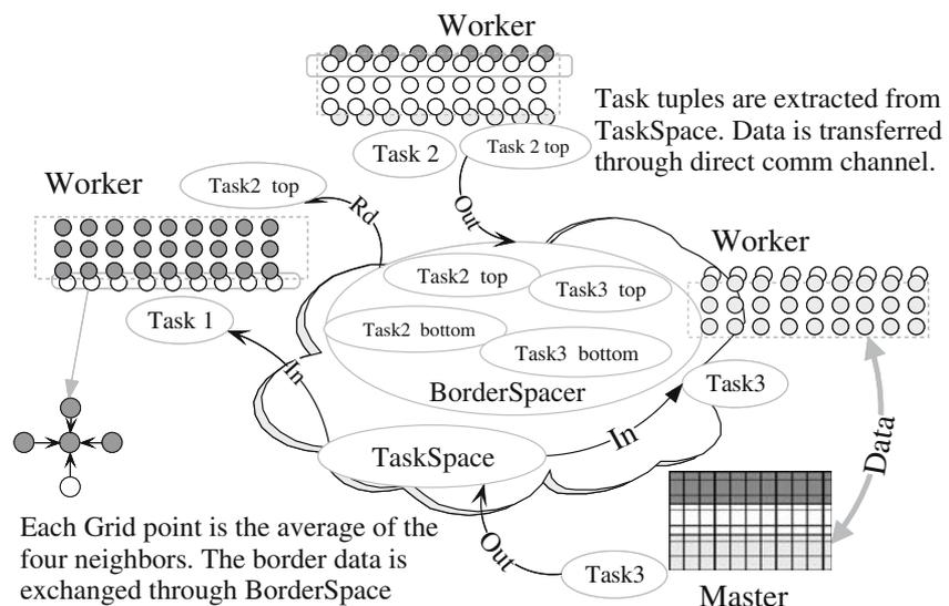
**Figure 8.** Operation of master and worker nodes for the CometG-based implementation of the heat distribution problem
