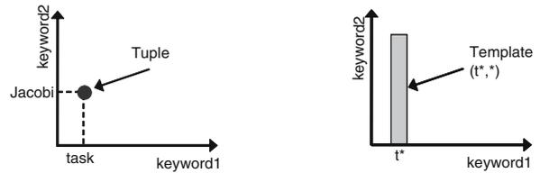
**Figure 2.** Example of tuples, templates and the semantic information space in CometG
